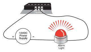
Figure 1: Relay output connected to alarm
