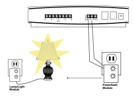
Figure 2: X10 Lighting Control Setup
