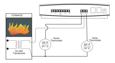
Figure 1: Dual Thermostat Setup
