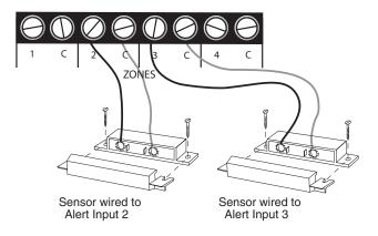
Figure 2-7 Two Sensors Wired to Adjacent Zones
