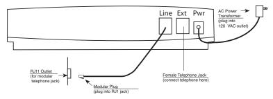
Figure 2-4. Installing the Telephone Line
