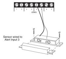
Figure 2-6. Sensor Connected to an Alert Zone
