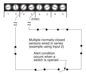
Figure 2-8. Multiple Normally Closed Sensors
